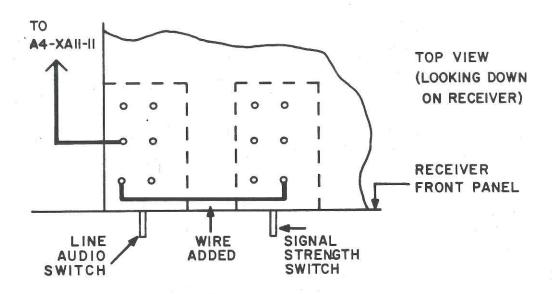
Figure 1-1. FSK Meter Modification
