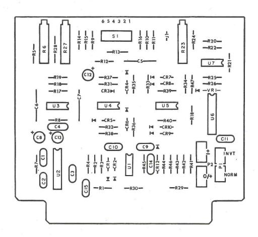
Figure 1-3. FSK Demodulator Parts Location
